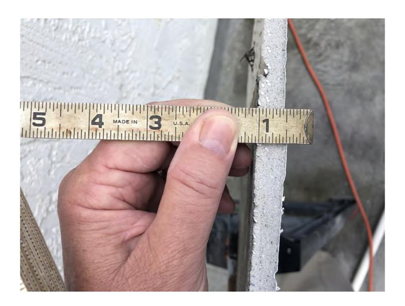
2 Inch lath lap - No cracks. Metal pristine. Metal shiny like new where cut through sample.
