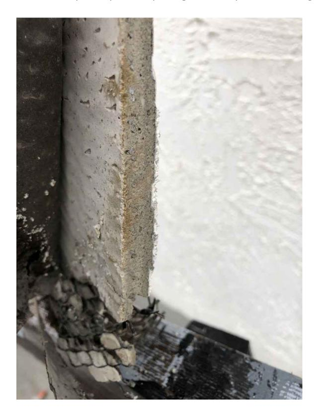
Stucco Cladding 1/2" Thick - applied using South Florida Building Code requirement or using the ASTM "unless otherwise specified" provision. No cracks anywhere. Metal shiny where cut through sample.
