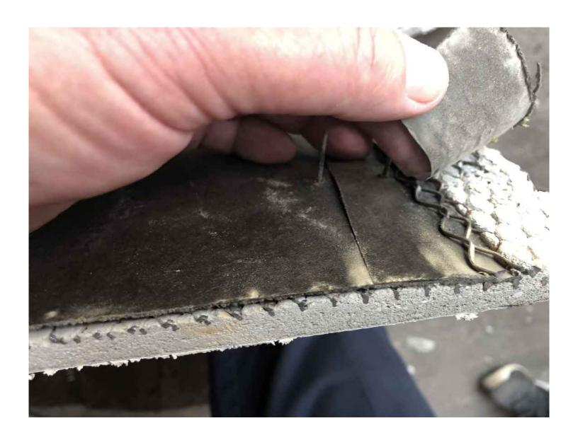
Un-Galvanized metal lath, no rust, no degradation, no water stains, no moisture deterioration. Just like the day it was put on 35 years ago. Constant weather exposure in Florida's environment. Lap is paper over metal. Still no Cracks, No faults, No flaws. Note: Crack seen in section sample underneath in rubbish pile was broken during removal.
