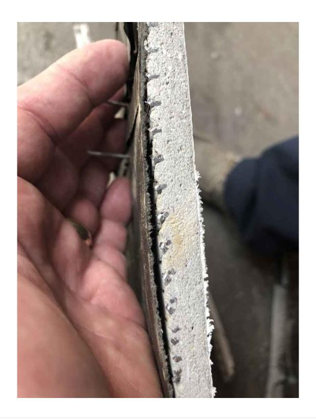
Un-Galvanized metal lath, no rust, no degradation, no water stains, no moisture deterioration. Just like the day it was put on 35 years ago. Constant weather exposure in Florida's environment.
