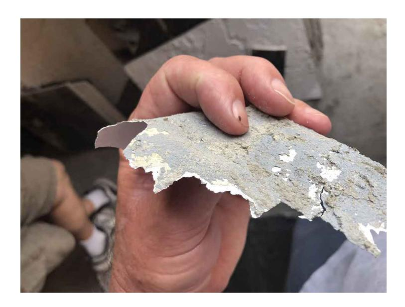
Stucco Cladding painted twice in 35 years, original paint and white re-paint. Both followed standard painting instructions and was applied with rollers to the standard mill thickness required by the manufacturer.
