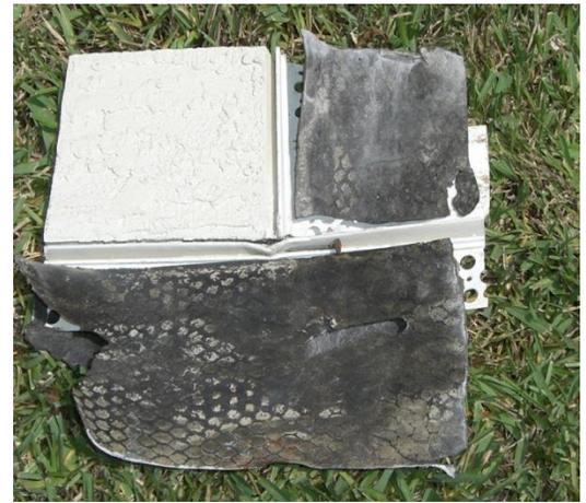
The photos above show the plastic control joint suffering the same fate as the expansion control joint - in order to make the lath discontinuous, the control joint was installed first and the paper lapped over.
